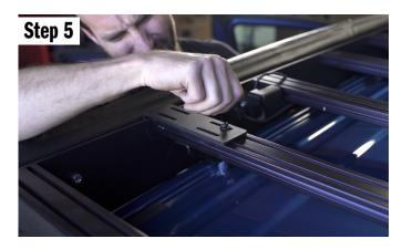
With the mounts in place, put a washer on the included black  $\frac{1}{4}$ " bolt, push it through the mount and thread it into the t-nut in the crossbar. Do this for all four locations on both brackets. Snug up the hardware, but leave it loose enough to adjust.
