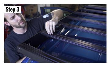
Now we need to prep your roof rack. You need to pick the two crossbars that you want to install the awning to. These locations can change based on the location of additional accessories on your rack. The best practice is to spread the two mounts apart as far as possible to spread out the awning weight. Once you pick your two crossbars, install 4ea drop-in style t-nuts in each crossbar. You will put two in the left track and two in the right track, trying to mimic the pattern on the mounts.
