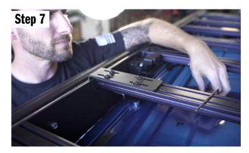
Next we can adjust the depth, move the awning as close to your rack and vehicle as desired. Then tighten the  $\frac{1}{4}$ " bolts on the top of the mounts. You are all set!
