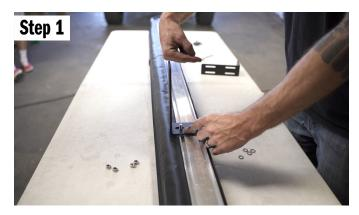
To begin our installation, we need to install the awning mount to the awning itself. Your awning should come with installation hardware that fits the T-Slot framing it has. You will first need to install those studs or nuts. Then we can position the mount. It can be installed as shown for the awning to sit beside your roof rack. Or, the bracket can be flipped 180 degrees to have the awning above the rack, allowing 360 degree lighting to still function.
