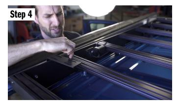
Next we need to lift the awning in place. This is best done with a helper, so you don't damage your vehicle. Adjust the mounts on the awning, so they line up with your selected crossbars.
