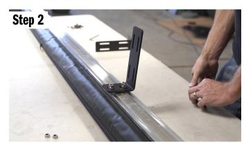
Put the included hardware in place on the mounts. Then tighten the hardware until it is snug, but still allowing you to adjust the bracket's location.
