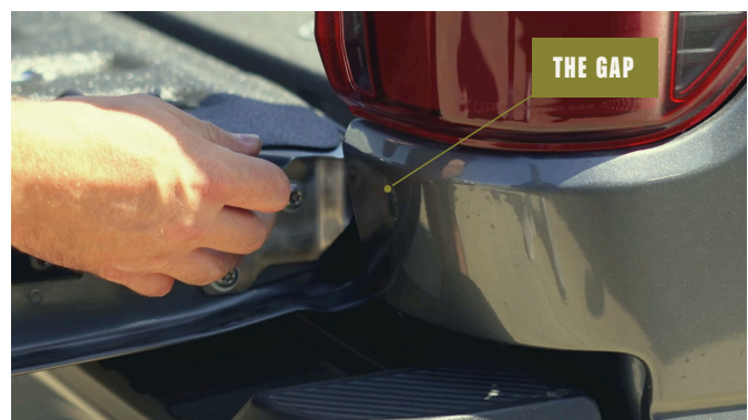
BOTH BOLTS STARTED, GAP SET, NOTHING TIGHTENED YET
