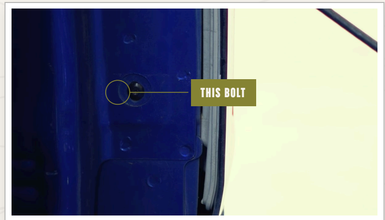
BED-END JAMB, BOLT STILL IN
