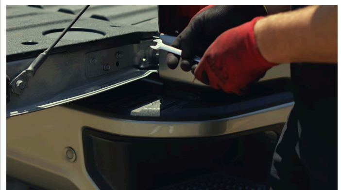
BREAKING THE FACTORY BOLTS LOOSE
