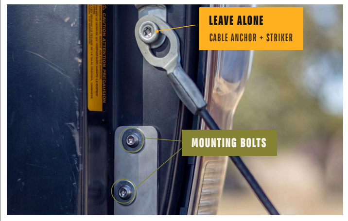
SHOWN INSTALLED – THE TWO SECURITY BOLTS SIT IN THE FACTORY BOLT LOCATIONS
