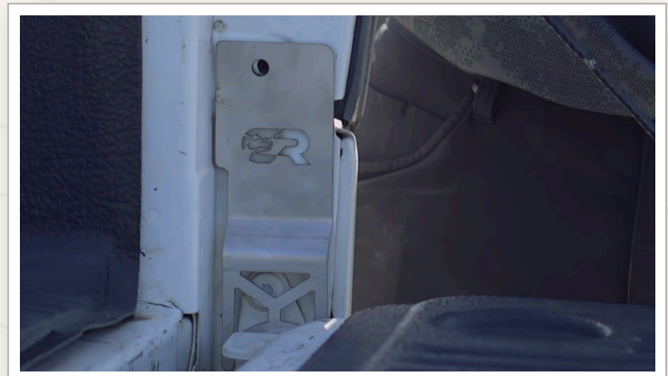
FLANGE FLAT ON THE JAMB, SHIELD LEG OVER THE HINGE
