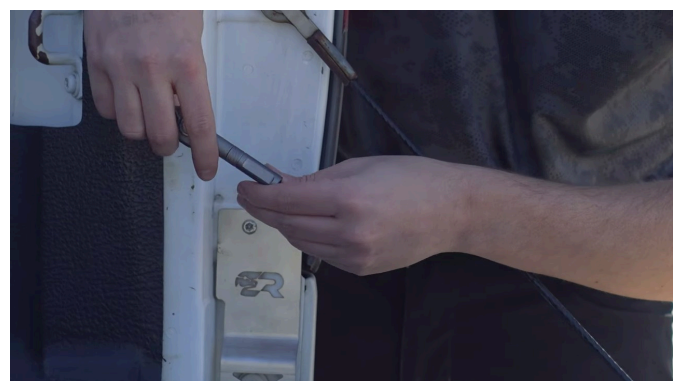
A – DRIVER AND BIT COME TO THE BOLT
