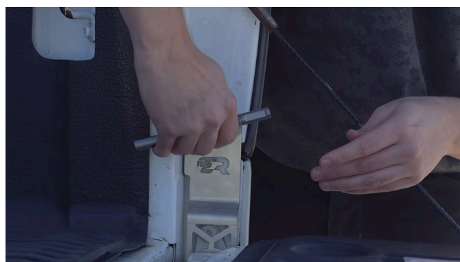
B – TIGHTEN UNTIL THE PLATE SITS FLAT
