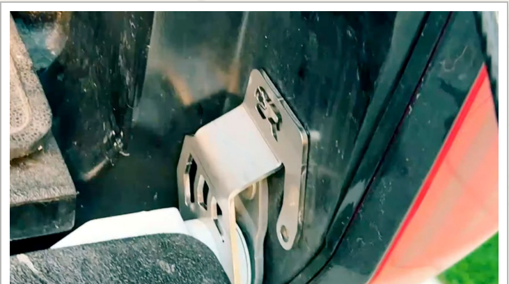
TAB FLAT ON THE PANEL, SHIELD OVER THE HINGE
