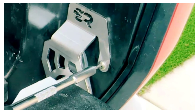
B — INCLUDED SECURITY BIT ON THE BOLT
