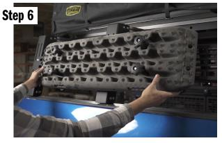
Now that the recovery boards are in place, adjust your mounts left to right. Using your 3/4 " wrenches, tighten the mounts to the bed rack. Then adjust the recovery boards up and down (only for boards that are in the green slots). With the boards in the desired position, tighten the pins/bolts to the mounts.
