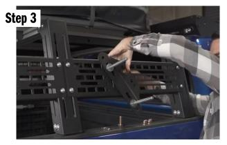
Now we will install the mount to your bed rack. Grab a gold (grade 8) bolt and put on a washer, then put that bolt through the mount, the same side as the pins. Use the inner holes. Line these up with the slots on your bed rack.
