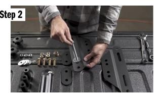
To use the included hardware start by placing a large washer on the long  $\frac{1}{2}$ " bolt. Push the bolt through the mount, so that the head of the bolt is inside the chanel, as show in the picture. Then place another washer on the bolt, then thread a nut all the way down. Snug the nut so it is not flopping around, but can be adjusted in later steps. Do this for all 4 locations on both mounts.
