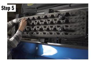
With the mounts up, we will now put our recovery boards on the mounts. Slide them over the pins. Then install the plastic spacer and knobs in all 4 positions. Tighten these so the boards are firmly attached to the mounts.
