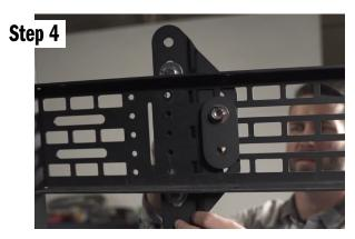
Next grab the oval backing plate and slide it over the bolt, then install a washer and lock nut. Do this for both positions, and on both mounts. Tighten these until they are not floppy, but still able to be adjusted.
