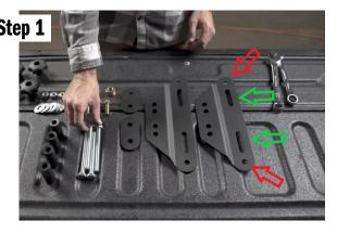
First we need to install the mounting pins for the recovery boards. You can use the included hardware, or the pins sold by the various recovery board brands. For Maxtrax install your pins/hardware at the RED locations. For all others like Tread or Amazon use the GREEN.
