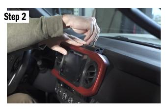
Using a #10 or 3/16 drill bit, push it into each hole on top of the mount and spin it clockwise to mark the center of the hole in your dash trim.
