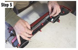
Set the drill guide onto position. THE HOLES IN THE DASH MOUNT ARE NOT SYMMETRICAL. It is important that the drill guide is put in position so that you can read the word "FRONT" and the arrows are pointing towards the face of the trim piece. Grab one of your #10 screws and put it in the first hole, then line the drill guide up so that it is parallel with the back of your dash trim.
