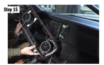
Note that the back of the mount has a groove for cable routing. You can slide a cable into this groove before installing the dash trim piece back in place.
