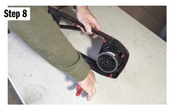
On the passenger side of the dash trim, where the  $\frac{1}{4}$  hole is close to the clip, you may need to very slightly trim the plastic so that your  $\frac{1}{4}$  bolt will fit in place.
