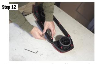
Tighten the two #10 screws and nuts with a  $\frac{3}{10}$  wrench and  $\frac{1}{10}$  allen wrench.
