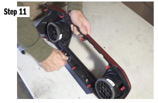
Tighten the four  $\frac{1}{4}$  bolts into position using a  $\frac{3}{16}$  allen wrench.
