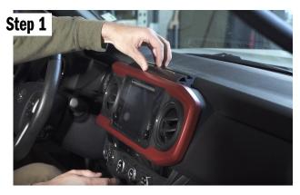
Set the dash mount on top of your dash and slide it to the drivers side until it stops, then move it to the passenger side approx 1/16 of an inch.
