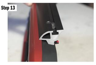
To install your mounting ball, first slide in a t-nut with the dimple facing down.
