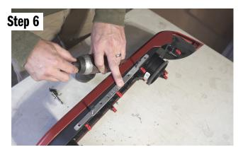
Drill the second #10 hole and put a bolt in that position to hold the drill guide in place.
