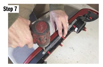
Drill the four 1/4 holes in the drill guide.
